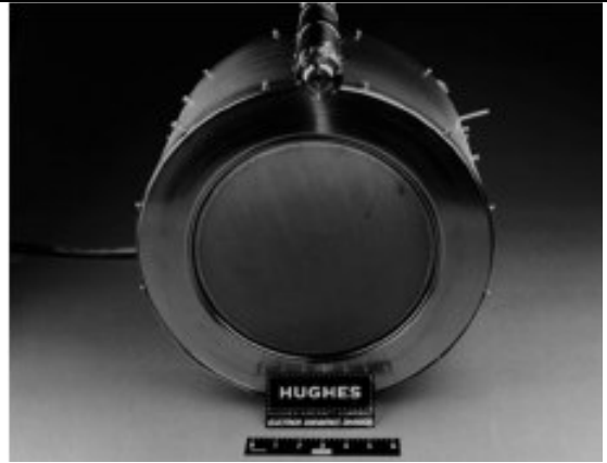
Figure 1.2: Electron Bombardment type electrostatic thruster 1
